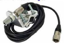
For mounting VLC5744 CB radio aerial to a horizontal pole, such as a mirror bracket. Constructed from high strength 5mm aluminium. Fits 15mm – 30mm diameter tube. Complete with 3m patch cable
