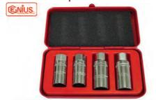
This ½" drive AF stud puller set allows you to remove studs without damage to surrounding machinery. The harder you turn, the harder they grip so you can remove even the tightest of studs. Made from chrome vanadium steel and presented in a sturdy metal case. Sizes: 1/4, 5/16, 3/8 and 7/16" (Box: 190x100mm).
