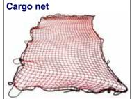
This 2.5m x 1.6m knotless net is made from high strength, fray resistant 3mm Polypropulene. With reinforced edging. A bungee cord around the edge for securing to trailer hooks.
