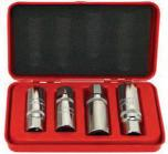
This ½" drive metric stud puller set allows you to remove studs without damage to surrounding machinery. The harder you turn, the harder they grip so you can remove even the tightest of studs. Made from chrome vanadium steel and presented in a sturdy metal case. Sizes: 6, 8, 10 and 12mm (Box: 190x100mm).
