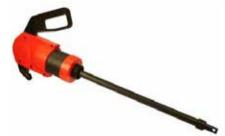
Polypropylene / alkathene polymer pump. Suitable for most liquids stored in standard plastic drums. The telescopic intake pipe will suit 100ltr and 250ltr drums and storage tanks up to 900mm deep. Delivery 330ml per stroke.
