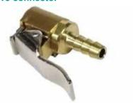
Snap on connector. Fits all standard 5 x 14mm tyre vales. Suitable for 6.35mm bore pipe.
