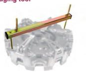
When rebuilding and fitting a dual clutch assembly it is important to ensure that the clutch release levers are correctly set. This bridging tool allows quick and simple height alignment of all levers so preventing premature release bearing or clutch plate failure. For Massey Ferguson.
