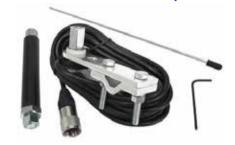
To enable optimum performance of CB when fitted to vehicles with cabs and bodywork constructed with high fibreglass content. Rigid 5mm aluminium construction. Fits tubes 15mm – 30mm diameter. Complete with 3m cable.
