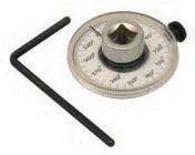
Designed for use on engines when an additional angular rotation movement is specified after torque loading is achieved can be used with any ½" drive wrench.
