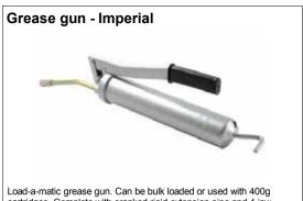
Load-a-matic grease gun. Can be bulk loaded or used with 400g cartridges. Complete with cranked rigid extension pipe and 4 jaw coupler. Operating pressure 705 bar. For replacements use, VLB1040 rigid pipe and VLB1018 couplers.
