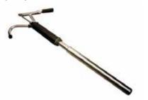
Hand lever operated metal barrel pump. Telescopic suction tube permits operation on barrels from 490mm to 865mm deep. Standard 2in BSP thread. Delivery 260ml per stroke.
