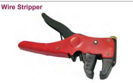
Automatic wire stripper with adjustable pressure jaws and wire cutter, suitable for stripping 25mm of 0.2 - 6mm diameter cable in one action.
