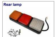
Complete LED modular rear combination lamp with stop/tail, indicator and reverse functions. Rubber base, Varivolt 10-30v, Length 275mm Width 95mm Depth 35mm. Replacement stop/tail module VLC2317. Replacement indicator module VLC2309. Replacement reverse module VLC2318.
