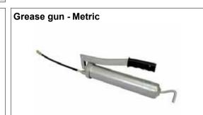
A Metric Load-a-matic grease gun. Can be bulk loaded or used with 400g cartridges. Complete with 30cm flexible extension pipe and 4 jaw M10 coupler. Operating pressure 705 bar. Use VLB1027 couplers and VLB1029/VLB1041 flexi pipes as suitable replacements.
