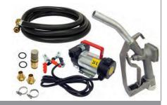
A self-priming pump with built in by-pass for diesel and light oil transfer. 40 litres per minute capacity. Supplied with on/off switch, carrying handle, 2m battery cable with clips, 4m hose, metal nozzle and filter. Requires 12 or 24 volt DC supply.
