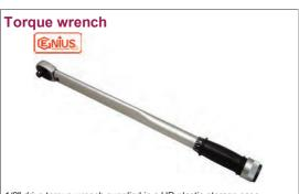
1/2" drive torque wrench supplied in a HD plastic storage case. Ergonomically moulded handle for added comfort, grip and durability. Capacity: 50-250 ft-lb (67-338 Nm). Length: 645mm.
