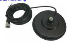
5" superior low profile Multipolar magnetic mount, 5m of 98% shield ultra low loss coaxial cable with PL-259 plug. 3/8x24T aerial fitment for VLC5744 3m Patch
