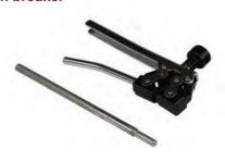
A simple and effective means of breaking roller chain. Simply place the chain into the device and tighten until the pin is removed. Large chain breaker - for chain pitch in range from 1" to 1 1/2".
