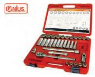
1/2" drive set in a HD plastic case. Including 27 12-point hand and deep hand sockets from sizes 3/8" to 1 1/4" and 3/8" to 7/8" respectively, a two way adapter (3/8" female to 1/2" male), 5" and 10" long extension bars, universal joint and a quick release ratchet.
