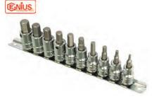
3/8" drive set with a wall mountable steel socket holder, this 10 piece metric hex bit socket set contains sockets 3mm, 4mm, 5mm, 6mm, 7mm, 8mm, 9mm, 10mm, 11mm and 12mm. Made of high speed tool steel.
