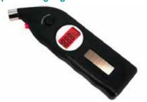
A neat palm sized tyre pressure gauge with a multitude of functions. Psi,Bar,kPa and Kg/cm2 can all be accurately measured under practical LED illumination. In addition to the integral tyre depth gauge, it is dual powered via an integral solar panel or 3V CR2032 lithium lon batteries in dim light. Autopower-off function maximises battery life.
