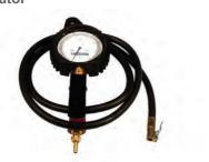
Airline inflator for standard bore valves. Calibrated 0.7 - 12 bar. Approved model according to European directive CEE 86/217.
