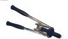
Industrial compound action hand riveter with high leverage long tubular steel handles. Head with nozzles to accept 3.2m 4.0 and 4.8mm aluminium alloy, stainless steel blind rivets.
