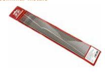
3.15mm diameter. A heavy coated rutile type all position austenitic ferrite electrode with a ferrite content of approximately 15%. 10 rods per pack
