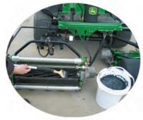
Back Lapping Compounds are ideal for sharpening cylinder mower blades in situ. Depending on the degree of wear and type of equipment the correct grade is available from fine to coarse. A stable, easy-to-use fluid which has low environmental impact and excellent value for money.
