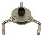
This clever little oil filter wrench attaches to a 3/8" drive ratchet handle and the design allows for broad range and tremendous gripping power. Fits easily into tight spots and features heavy duty grooved legs for a more positive grip. Fully adjustable from 65-110mm (2 1/2" - 4 5/16").
