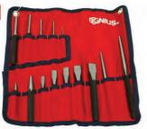
Contained in this handy canvas tool roll is: 3 and 5mm centre punches; 6, 10, 12, 14 and 16mm flat chisels; 3 and 5mm long taper line up punches; 2, 3, 4, 5 and 6mm pin punches. All are made from high speed tool steel and are ideal for even the most demanding of tool users.
